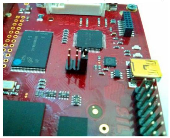
Pengwyn takes the power from the mini-USB connector CN6 and/or connector CN1.
