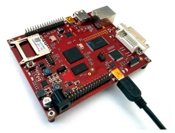
which you can connect, by means of a mini-USB cable, to your personal computer.
